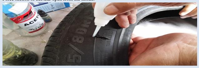
Pour Satlon 105 over both edges making sure that the glue penetrates right through the cut to the inner surface. (please take note of just where the cut/tear is as im going to show you the end result soon and you may be surprised at just how well this works)
