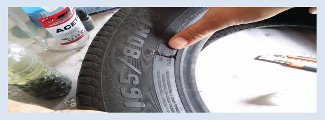
Now give pressure making sure that it is constant and the cut/tear is closed completely. The amount of time should not be less than one minute worth of pressure. I have personally tested this at 16 seconds and went straight to 4 bar pressure. (Something I would not advise you to do as this is in fact a stupid and meaningless exercise when you and your families lives are at stake) one minute or more should be sufficient.
